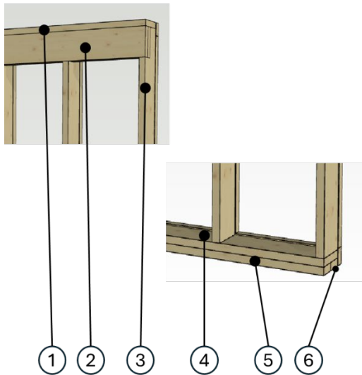
FIGURE 4B— ILLUSTRATION OF TYPICAL WALL PANEL VERTICAL TOP PLATE
