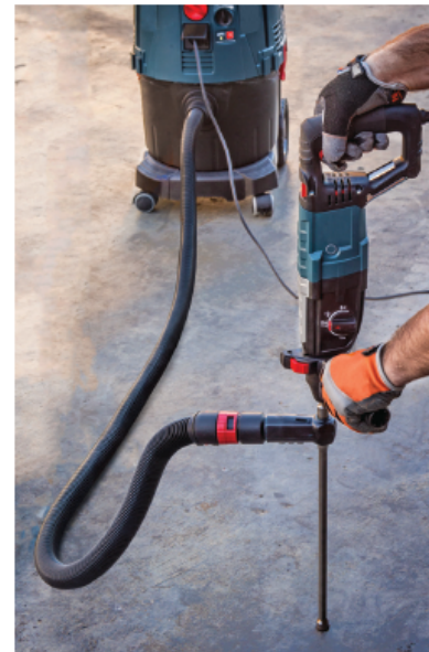
Bosch/Simpson Strong-Tie DXS drill bit used with the vacuum dust extraction system described in Section 3.2.3.2
