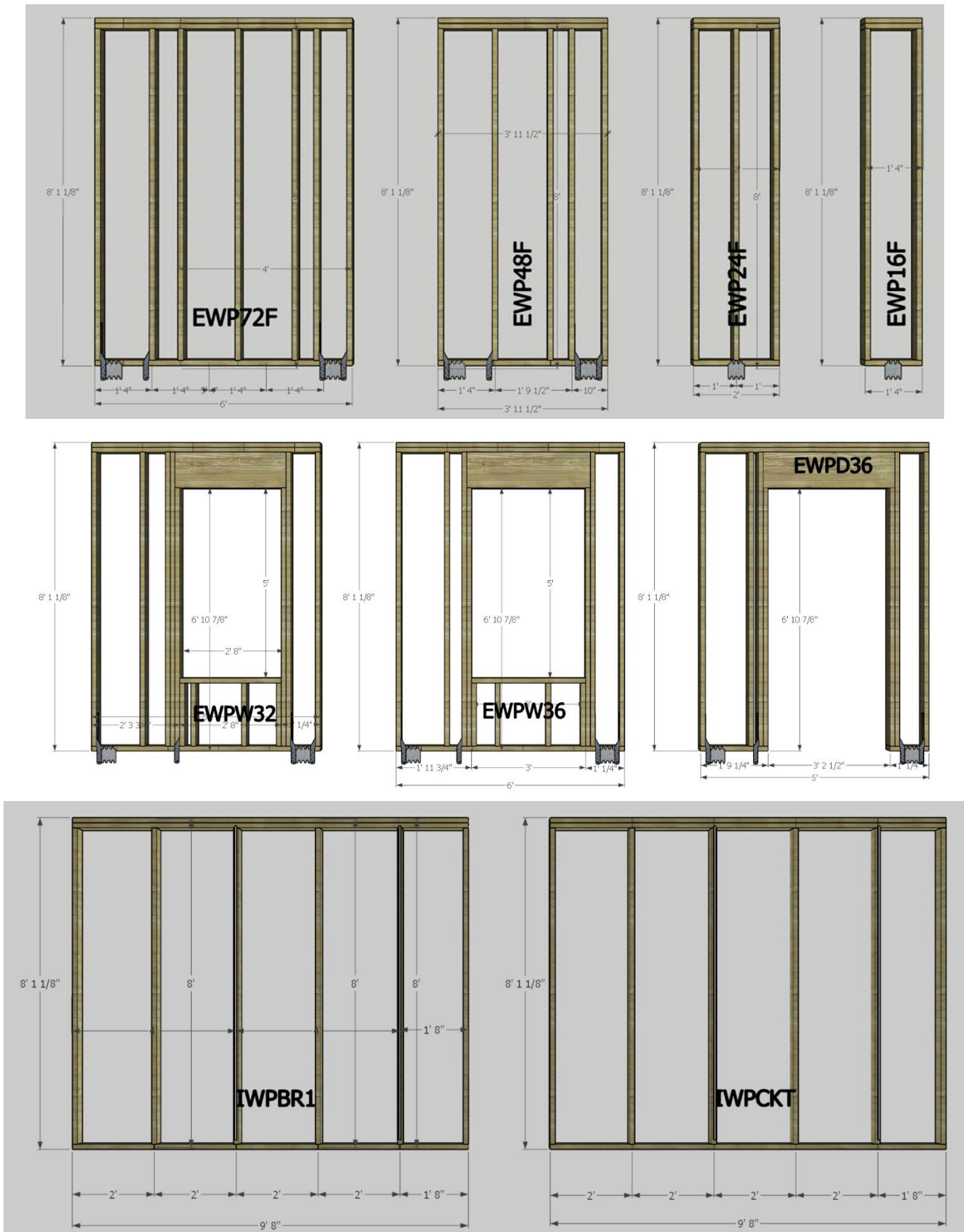
FIGURE 4—WALL PANELS WITH IDs
