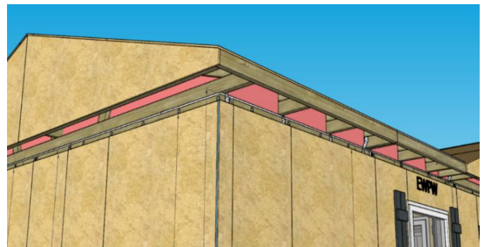
4). Roof/ceiling panel connection perpendicular to wall
