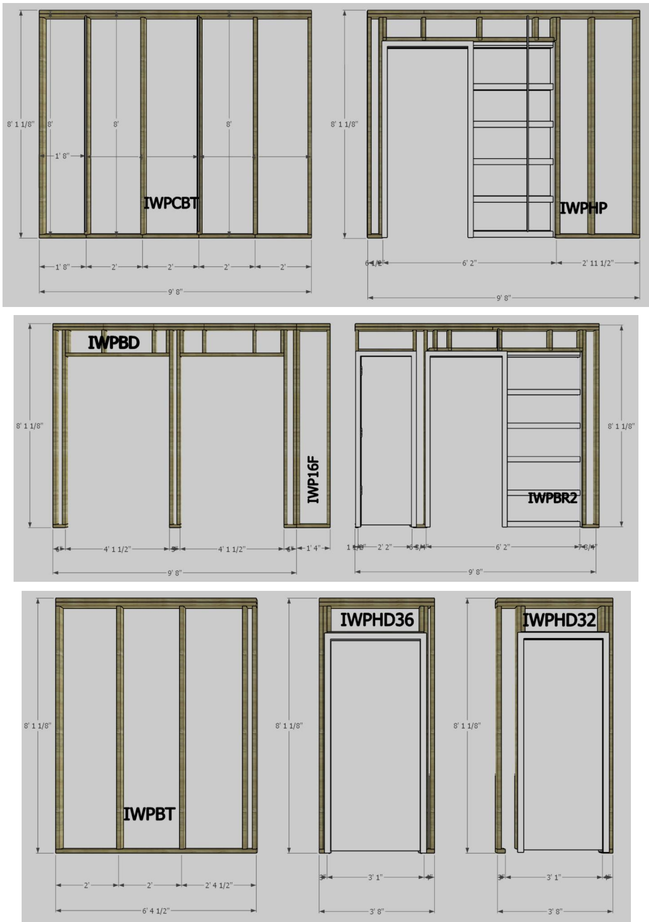
FIGURE 4—WALL PANELS WITH IDs (CONTINUED)
