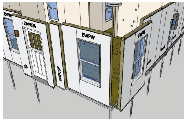
2). Exterior Panels EWPW and EWP16F installed in line
