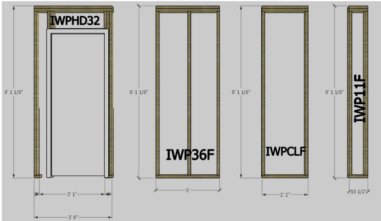
FIGURE 4—WALL PANELS WITH IDs (CONTINUED)
