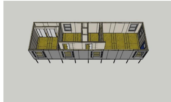
4) Interior wall panel installation
