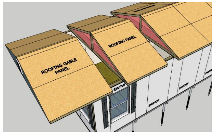
2). Roof/ceiling panel to panel schematics
