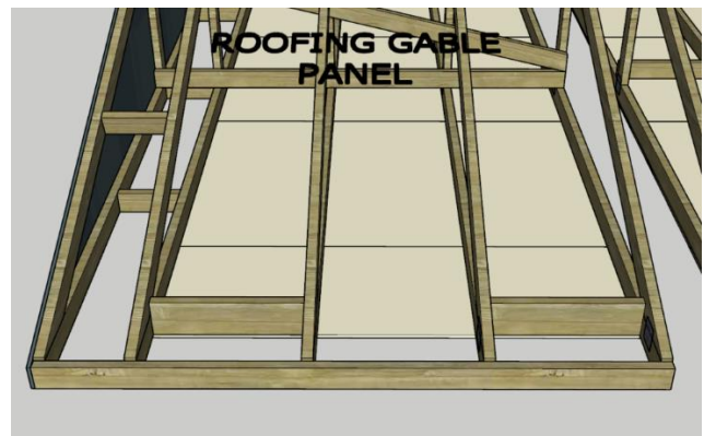
6). Blocking at roof/ceiling panels
