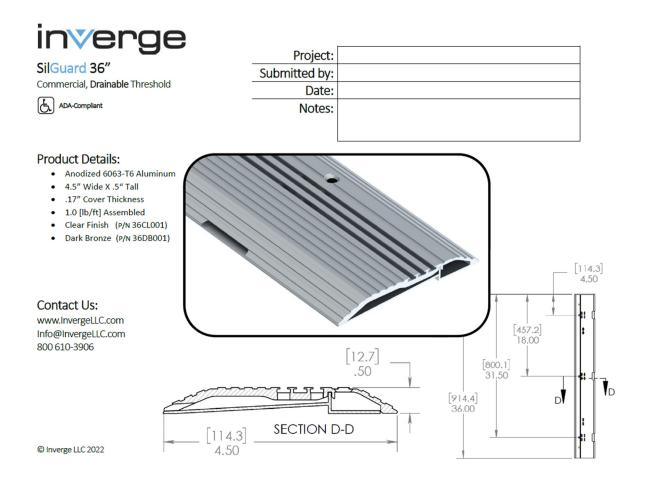
FIGURE 1—SILGUARD DRAINABLE THRESHOLD
