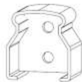
FIGURE 14—TOP AND BOTTOM RAIL BRACKETS FIBERON® CITYSIDE CONTEMPORARY ALUMINUM GUARDRAIL
