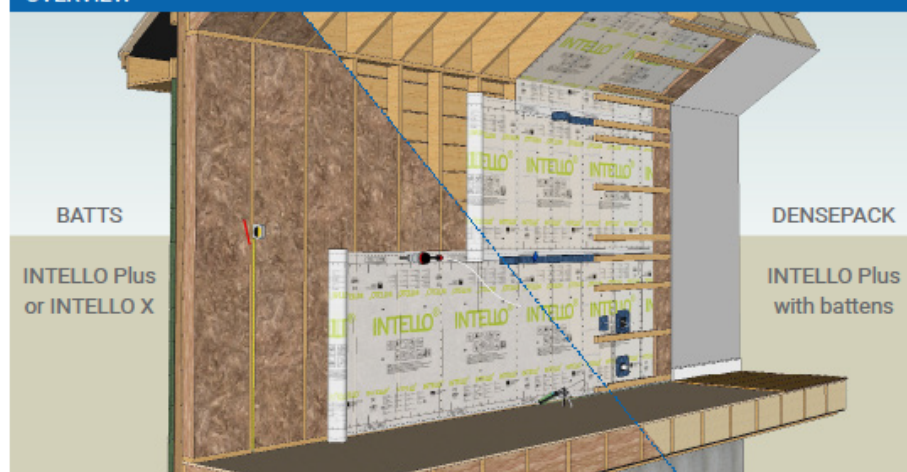
FIGURE 1—TYPICAL INSTALLATION OF INTELLO PLUS AND INTELLO X MEMBRANES
