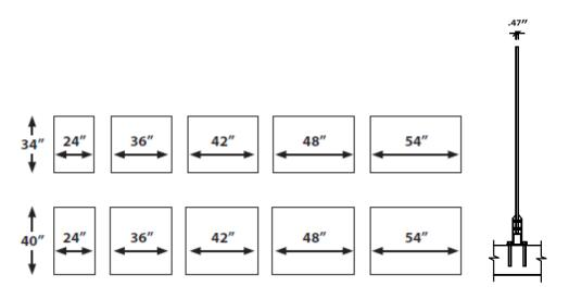
FIGURE 4—GLASS PANEL HEIGHTS AND WIDTHS
