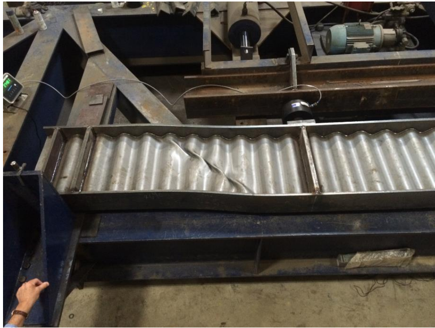
Figure 3 – Typical Shear Failure
