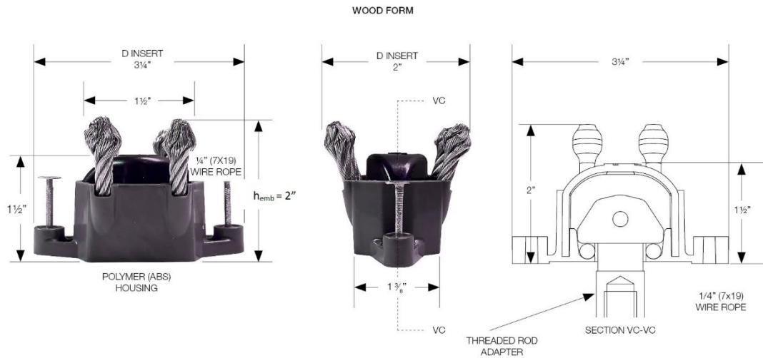
FIGURE 3B—LOW PROFILE SPIDER SX-WF-LP WITH THREADED ROD ADAPTER (SX-ADP) INSERT ASSEMBLY
