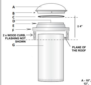
18", or 21" Diameter Plastic Dome attached during the manufacturing process to a 0.063-inch-thick aluminum frame (Alloy 1100, Temper 0, ASTM B209)
