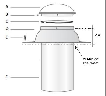
A - 10", 13", 18", or 21" Diameter Plastic Dome attached during the manufacturing process to an 0.063 inch thick aluminum frame (Alloy 1100, Temper 0, ASTM B209)
