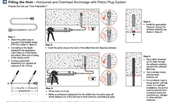
Note: Refer to Table F for proper gel times and cure times and Table D for maximum tightening torque.
