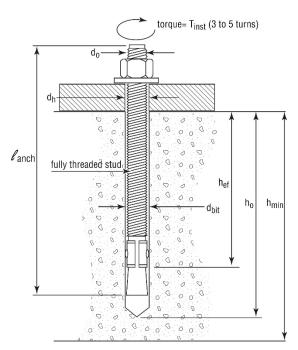
FIGURE 2—ITW RED HEAD TRUBOLT WEDGE ANCHOR (INSTALLED)
